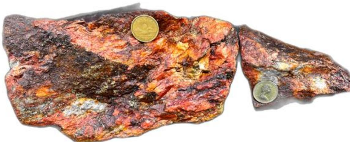
Greyish quartz vein with mineralization comprising of fine sulphides (chalcopyrite, bornite, pyrite and molybdenite).
