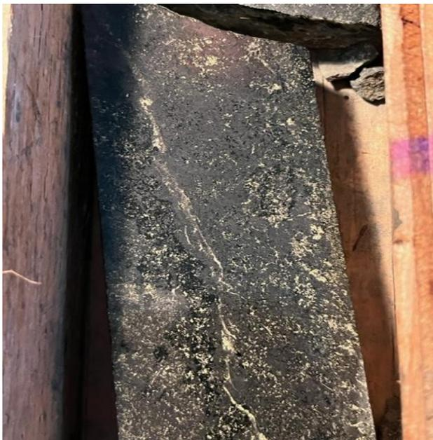
**Plate 1: Representative sample of drill core containing semi-massive chalcopyrite and gold in a garnet-epidote skarn in the northern portion of the MZM, Silver Hart**
